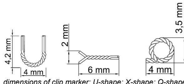
dimensions of clip marker: U-shape; X-shape; Q-shape
